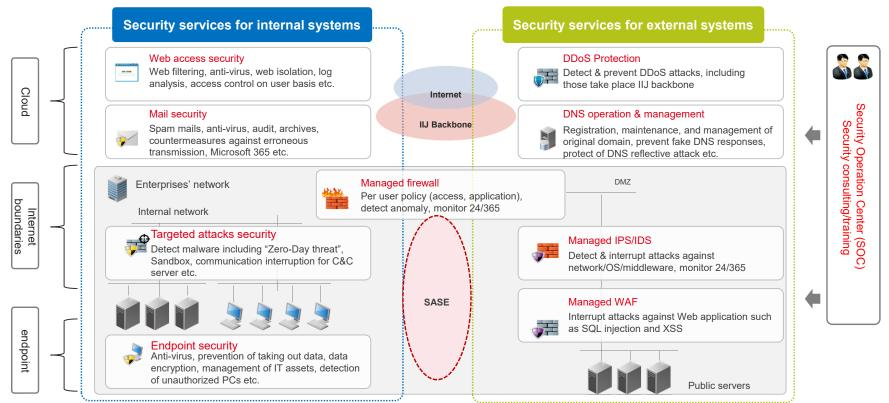
SASE (Secure Access Service Edge) is a concept to shift controls of network and security on the route to Cloud services to enable secure access from any points, instead of the conventional centralized management through headquarters or data centers
