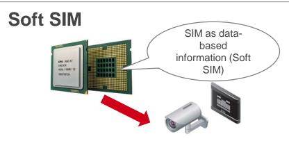
A communication module given SIM functions where the information required for mobile communications is logically written in internal memory
